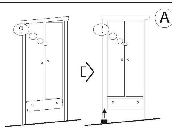
If one of the legs comes free from the floor or if the wardrobe is not standing at right angles, you will have to push a wedge or a sheet of paper plied in the desirable thickness, under the leg.
