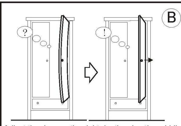
Adjust the door on the right depth using the middle hinge.
